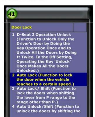
lever to P range from other than P range when the ignition is ON.)
